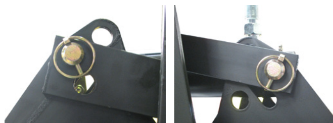
Synchronising links - Viewed from below
