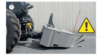
**CAUTION:** Always place the weight + MULTIBOX assembly flat. The weight must be hitched at 3 points. Automatic hitching risks damaging the MULTIBOX (7).
