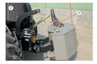
When 3-point hitching is used, if the automatic support makes contact with the arms when lifting, the bracket tilts forward to ensure full compatibility (4).
