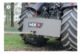
When towing, the pin (4) must be in the low position, to lock the tilt of the bracket.
