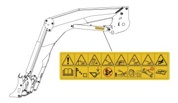
Safety stickers are affixed to the loaders. Ensure that these stickers are clean and legible; replace them if they become damaged. If replacing a sticker, clean the surface used for the sticker with isopropyl alcohol and affix the sticker using a special tool.
