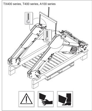
Ensure all parts of the loader are firmly bound together to remove it from the pallet (See loader unpacking instructions).
