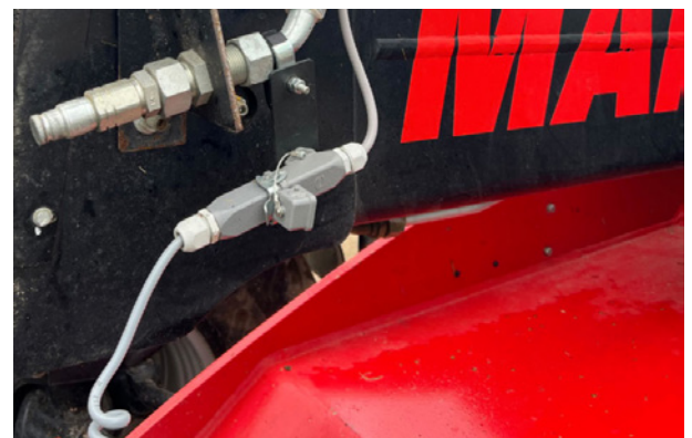
4th function electrical availability on a telescopic handler - to be adapted by the customer.
