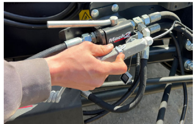
Electrically fitted for 4th function on silage feeding bucket. Original fitting on loader or telescopic handler side not supplied.
