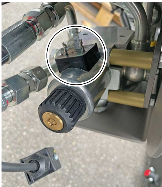
3rd function solenoid valve on the C400PRO loader.
