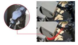
Built-in 7-pin socket, with a 3 m maleto-male spiral cable for a neat, secure connection.
